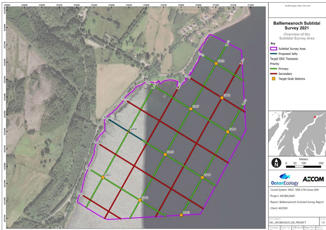
Figure 2-1: Grab sampling locations in relation to drop-down camera transects and proposed jetty location
